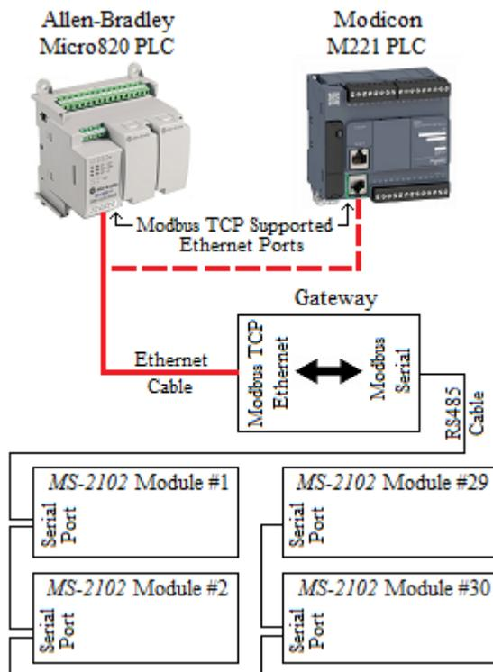
data stream to Modbus TCP Ethernet packets.
